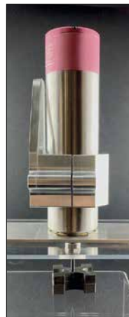
Figs. 5–6 CNC head to obtain a perfect surface finish on the green part
