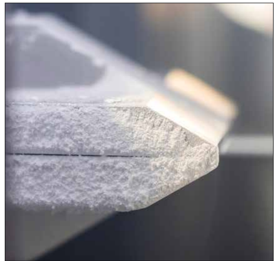
Fig. 3 Aerosol Deposition enables the formation of unique metal and ceramic coatings at room temperature on all types of material surfaces
