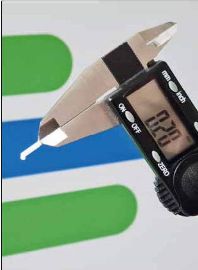
Fig. 5 The tubes, with sharp bends and inner contours, were defined and produced with minimum wall thicknesses of 200 \mu\text{m} , as well as perfect surfaces with roughness values of Ra_{\text{max}} = 0,4
