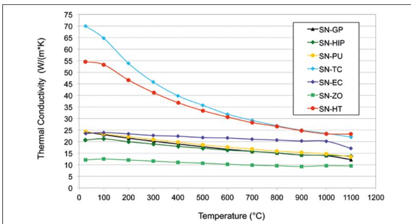
Fig. 4 Temperature-dependent variation of thermal conductivity for different silicon-nitride grades available at FCT
